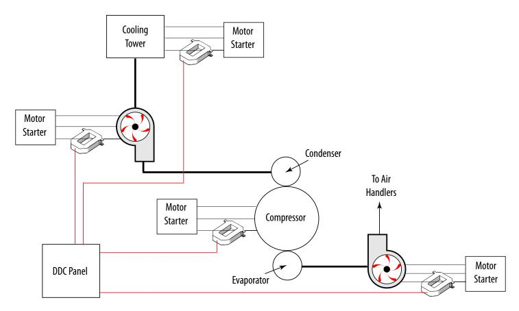
The total kW for the system is calculated by summing the kW values measured at each section of the chiller plant:
